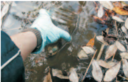
DO NOT sample in stagnant areas with little flow. DO NOT stir up bottom sediments or allow foreign materials to enter the sample bottle. (DO be careful to grab a clean sample in cases where stormwater runoff is shallow.) If the runoff is so shallow that it is not possible to sample without the sample being contaminated in the process, then find an alternative way to sample.
