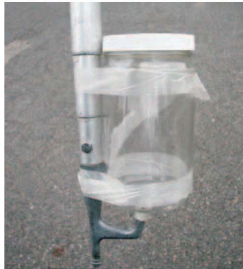
DO attach a bottle to a pole for sampling in manholes or when a hand sample would be in stagnant water. A boathook is used in this example and the bottle is attached to it with filament strapping tape.
