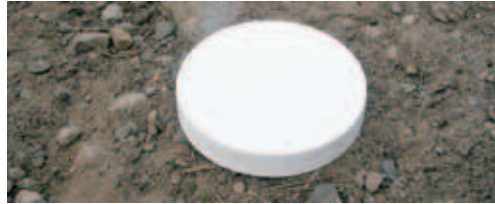
DO NOT allow bottle lids to touch ground. Keep lids clean to prevent contamination.
