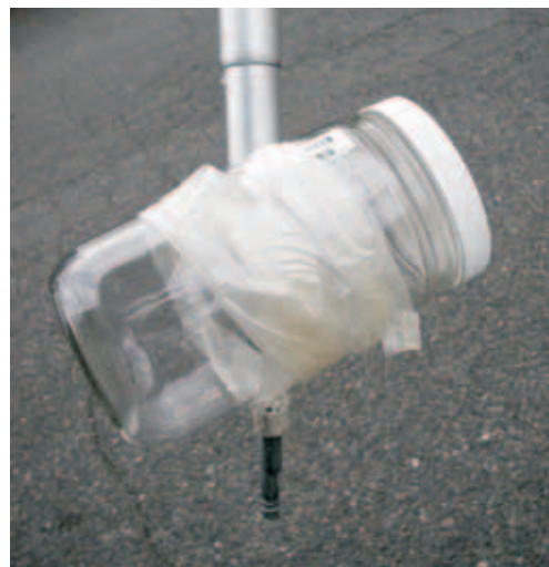
If the water is too shallow to sample with the bottle upright on the pole, try taping it on sideways, but tilted up slightly.
